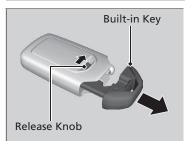
The built-in key can be used to lock/unlock the doors when the keyless remote battery becomes weak and the power door lock/ unlock operation is disabled. To remove the built-in key, slide the release knob and then pull out the key. To reinstall the built-in key, push the built-in key into the keyless remote until it clicks.
