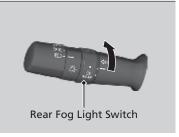
To turn the rear fog light on Rotate the switch to Oth. The Oth indicator comes on.
