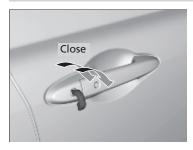
Lock the driver's door with the key. Within 10 seconds of returning the key to the central position, turn the key in the lock direction and hold it there.
