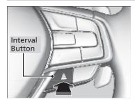
Press the interval button to change the ACC following-interval.
