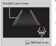
When the LKAS is suspended, the lane lines on the gauge change to double lane lines, and the beeper sounds (if activated).
