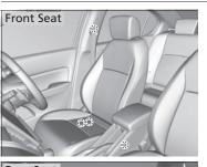
When replacing the seat belts, use the anchorage points shown in the images. The front seat has a lap/shoulder belt.
