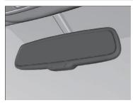
When you are driving after dark, the automatic dimming rearview mirror reduces the glare from headlights behind you, based on inputs from the mirror sensor. This feature is always active. Automatic Dimming Rearview Mirror\*
